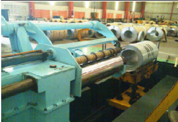
Exhibit 7. Cutting process for steel plate
